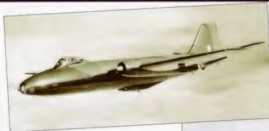
Above: The interdictor B(I).Mk 8 version could carry a belly pack of four ADEN cannon for strafing. Its main role, however, was as a tactical nuclear bomber.
